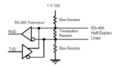
The figure shows how the terminating and bias resistors are used in a typical half-duplex circuit. If the serial channel is being used for RS-485 data transmission, an internal set of termination and bias resistors can be switched on the Tx/Rx signal pair. For
